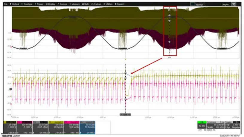
Figure 5. Phase current, leg current sensing signal, and OCPn signal. Experimental waveforms during switching cycles and a zoomed view. C5 grey 20 A/div is the phase current measured with an external current probe, C1 yellow 1V/div is OCPn, C2 pink 500 mV/div is the amplified leg shunt current signal. t = 50 ms/div, zoomed view t = 50 \mu\text{s}/div .
